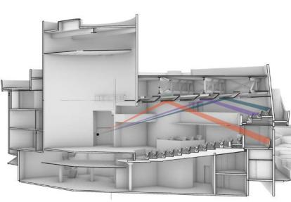
Acoustics Figure 23 Current Balcony and Audio Mix Ceiling Reflections - Midstage Source
