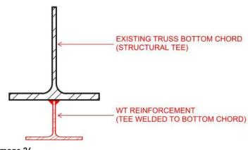
Image 26 Typical WT reinforcement detail
