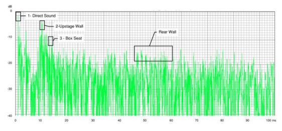
Acoustics Figure 10 Upstage center source to receiver F104 acoustic model and energy time curve
