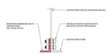
Image 25 Typical bolted reinforcement detail
