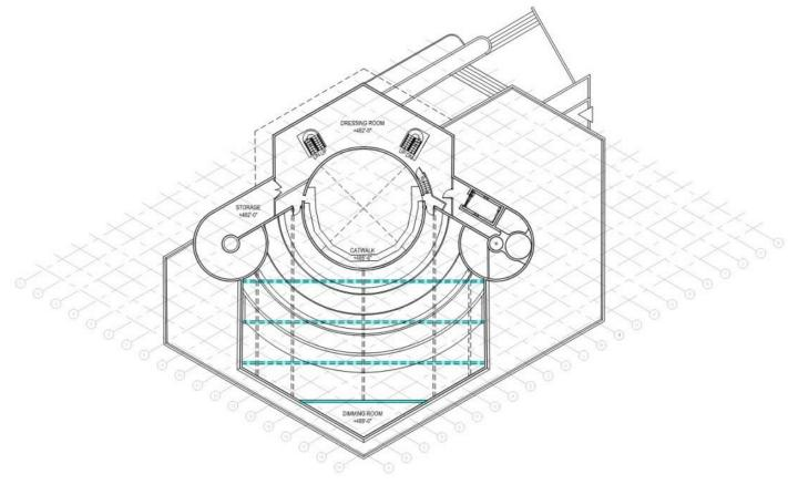
Image 24 Plan diagram with four primary roof trusses highlighted
