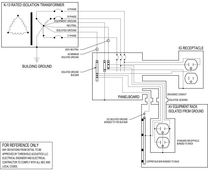
AV Figure 1 Clean Technical Power isolated ground typical wiring and distribution
