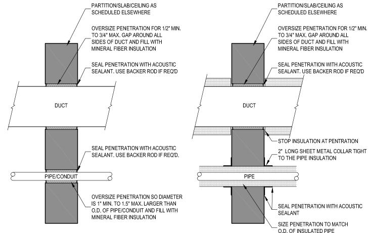
Acoustics Figure 41 Penetration details without (left) and with external insulation (right)
