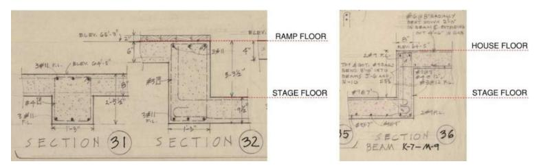
Image 19 Markup of original plans showing existing structural layout, slab steps and beams. Courtesy of Avery Library.
