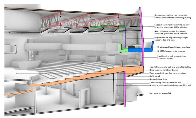
Image 15 Diagram showing proposed structural changes in house
