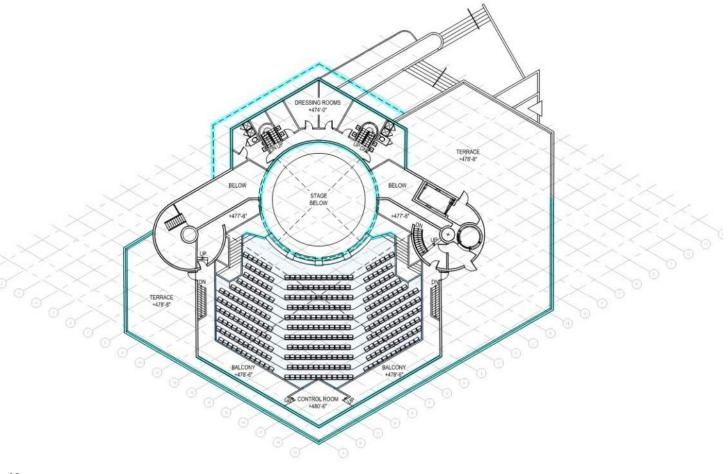
Image 18 Plan diagram showing extents of shoring required for removal of house floor highlighted in blue
