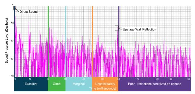
Acoustics Figure 4 Energy time curve labeling the impact of time of arrival on the ability to understand spoken word
