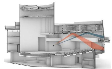
Acoustics Figure 22 Current Balcony and Audio Mix Ceiling Reflections - Downstage Source
