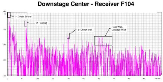
**Acoustics Figure 9** Downstage center source to receiver F104 acoustic model and energy time curve
