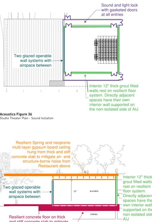
and stiff concrete slab to mitigate air- and structure-borne noise from Parking below
